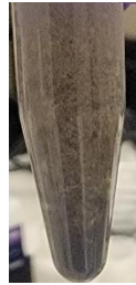
Image 1: Wastewater sample and LM carbon beads in RPSWB after tumbling for 4 hours.
